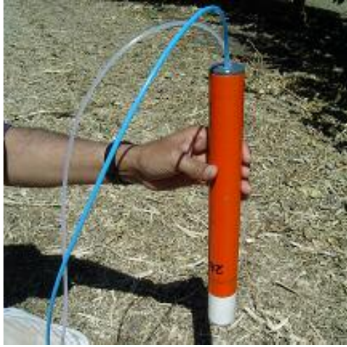
Figure 12: Soil solution extraction tube. Tubes are installed at varying depths to measure the amount of nutrients in the soil solution in the root zone and below the root zone. The tube pictured is manufactured by SARDI for the tri-state salinity project.
